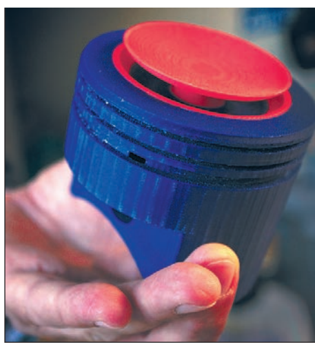
The Grail engine features a valve in the piston.
