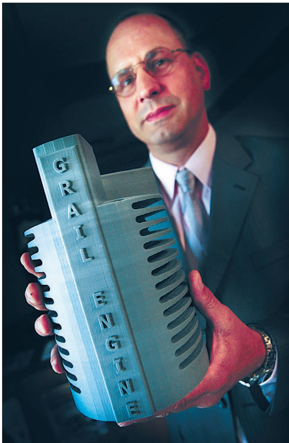
Photos by TOM DORSEY / Salina Journal Matthew Riley, CEO and chief research scientist of Grail Engine Technologies, holds a plastic model of an air-cooled cylinder of a Grail engine. A Grail engine could run on a variety of fuels, including gasoline, diesel, hydrogen, propane and natural gas.
